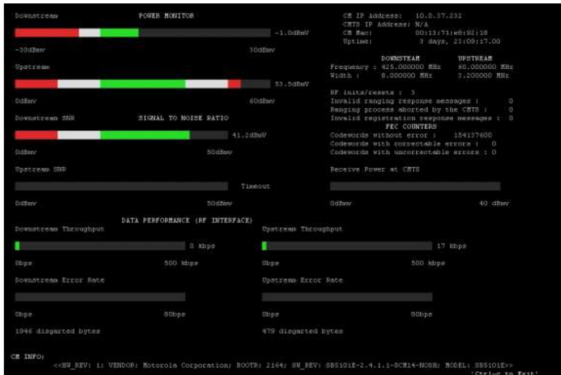
Figure 9 Real time modem monitoring [9]
