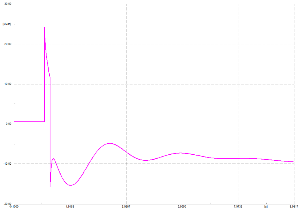
Figure 12. Reactive power of the 75 MW generator
