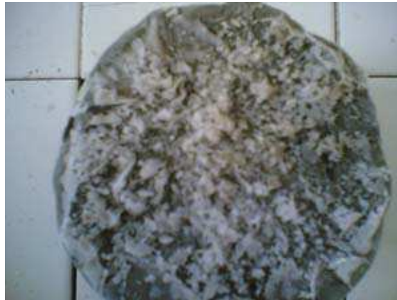
Fig. 1 Crystallization on surface after the freezing
