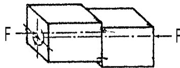
Figure 4. Friction welding including orbital movement [5].
