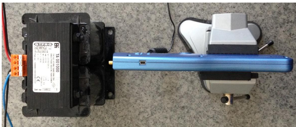
Fig. 3 Transformer and Magnetic Field Spectrum Analyzer
