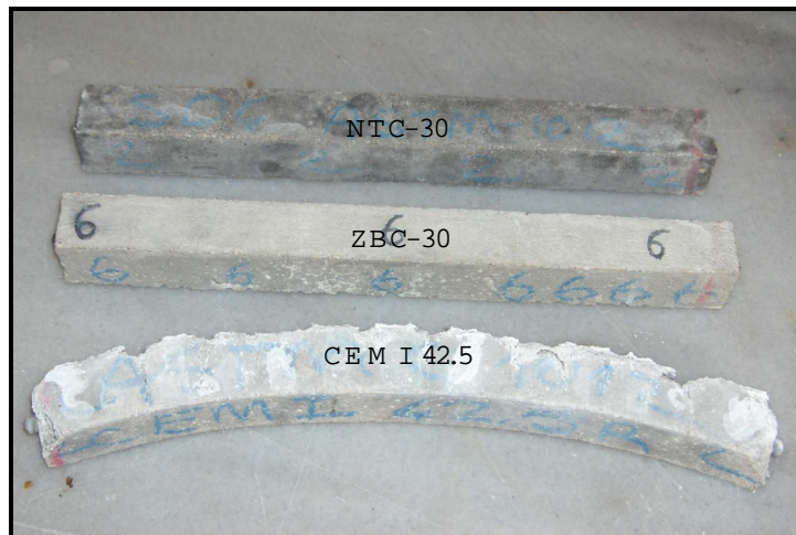
Figure 2: Physical deterioration of mortar bars at 6 months sulfate exposure.
