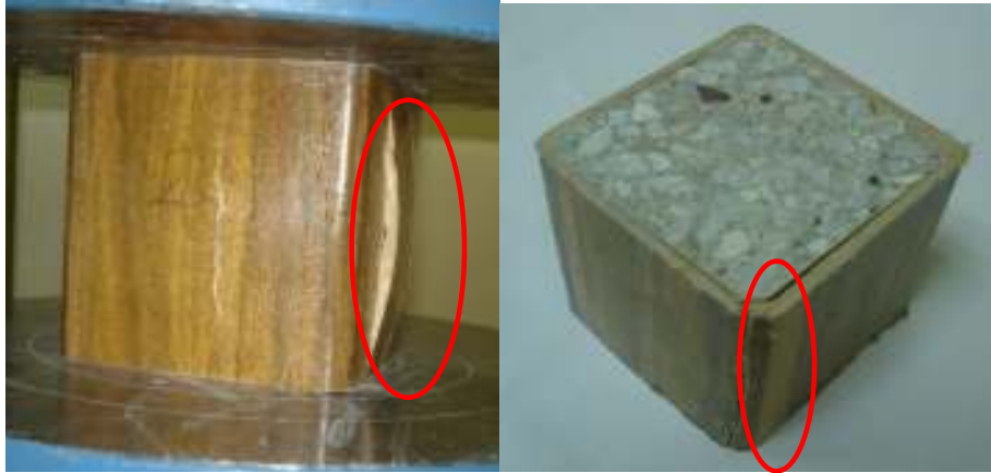
Figure 7: Concrete filled GFRP samples failure pattern
