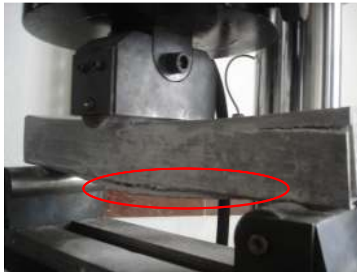
Figure 13: Beam Sample after Flexure Test
